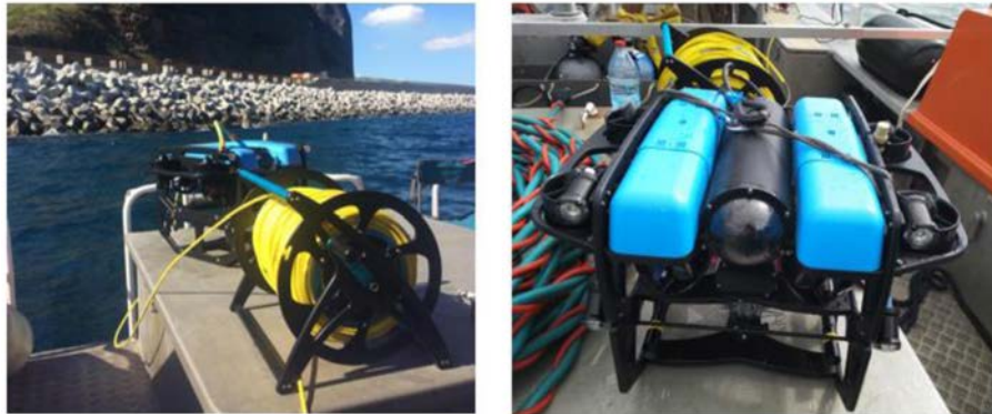
Figure 6—ID OCEAN mini-ROV on NRL seawall inspection
